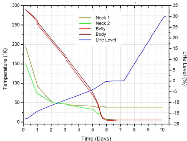
**Figure 11: Cooling the OSG using the Cryogenic refrigeration system.** It takes about 10 days to cool the OSG using only the Cryogenic refrigeration system and Helium gas. Initial experiments show this time will be halved to less than 6 days for the *iGrav*<sup>TM</sup>
