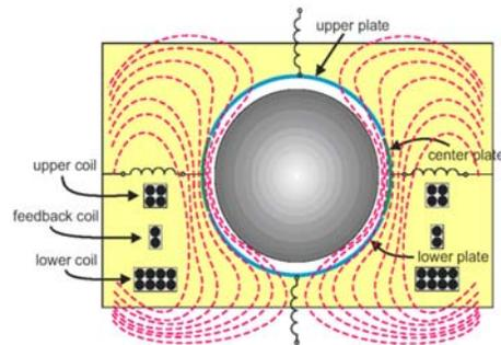
**Figure 5: Drawing showing magnetic flux distribution from Upper and Lower coils, In response to the magnetic field that results from the currents in the coils, currents are induced in the surface of the sphere that prevent flux from entering sphere. The interaction between the induced currents in the sphere and the currents in the coils produces the force that levitates the sphere.**
