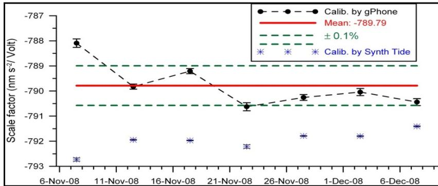
**Figure 1: Variability of gPhone Scale Factor.** Scale factor varies by more than  $\pm 0.1\%$  over a two month time span. (U. Riccardi et al. (2010A))
