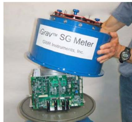
**Figure 4: Integrated data acquisition and control electronics.** Microprocessor-controlled electronics with A/D converter reside in Dewar head. Real-time controller for high-resolution data logging with 7.5 digit DVM for Gravity Signal and Barometer with GPS time stamp. Electronics are sealed in He gas and immune from atmospheric oxidation and humidity.
