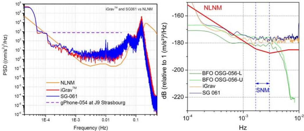
**Figure 9:** On the left side - Noise comparison of *iGrav*<sup>™</sup> and OSG061 compare to NLNM. On the right side - Noise comparison of *iGrav*<sup>™</sup> and OSG061 compare to Black Forest Observatory OSG-056 Dual Sphere SG and NLNM
