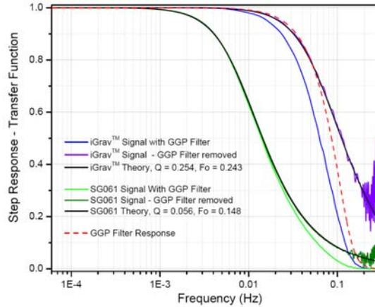
**Figure 8:** A comparison of the open loop transfer functions of the *iGrav*<sup>™</sup> and the OSG
