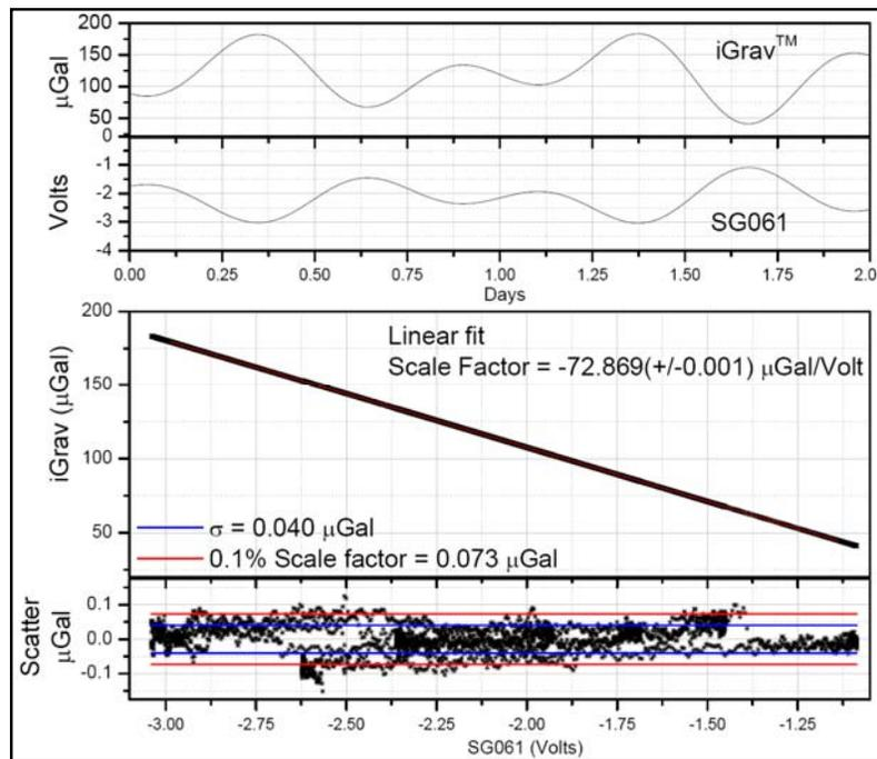
**Figure 10: First test of concept of using *iGrav*<sup>TM</sup> to “calibrate” other SGs** Note that the standard deviation of the scatter is  $0.04 \mu\text{Gal}$  when two SGs are least squares fit together. This compares to a standard deviation of about  $1 \mu\text{Gal}$  when an AG is fit to the SG. This suggests that using an *iGrav*<sup>TM</sup> to determine relative calibrations between SG sensors will be 25 times more precise than using an AG.
