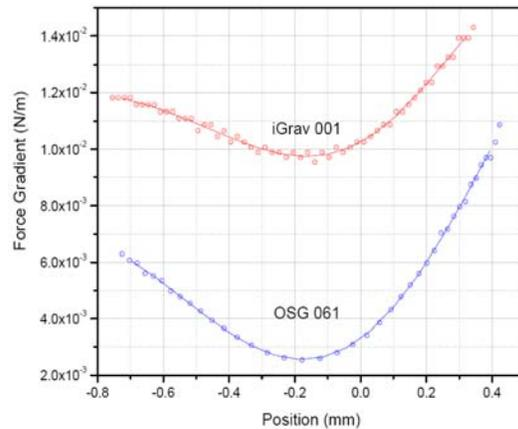
**Figure 7: Magnetic force gradient versus position: *iGrav*<sup>TM</sup> vs. OSG.** The X-axis is a measure of the sphere position with respect to the center of the capacitance bridge. The Y-Axis is the gradient (spring constant) measured in Newtons/meter.
