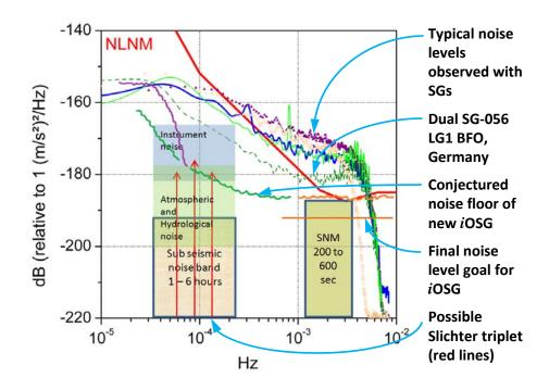
**The goal of the** *i***OSG** is to attain an instrumental noise level less than 0.3 (nm/s²)²/Hz, which is below the NLNM
