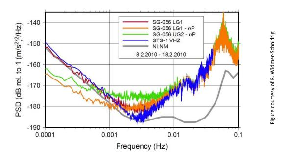
Noise spectra of 10 quiet days for OSGs at the Black Forest Observatory (BFO), Germany. SG-056 LG is the sensor with higher levitated mass, showing lower noise than the standard OSGs. The "-  $\alpha$ P" designation indicates time series with the gravitational effect of atmospheric pressure variations removed. Spectra of the BFO STS-1 long period seismometer and of the New Low Noise Model, based on the lowest noise ever observed by STS-1 sensors anywhere, are included for comparison.
