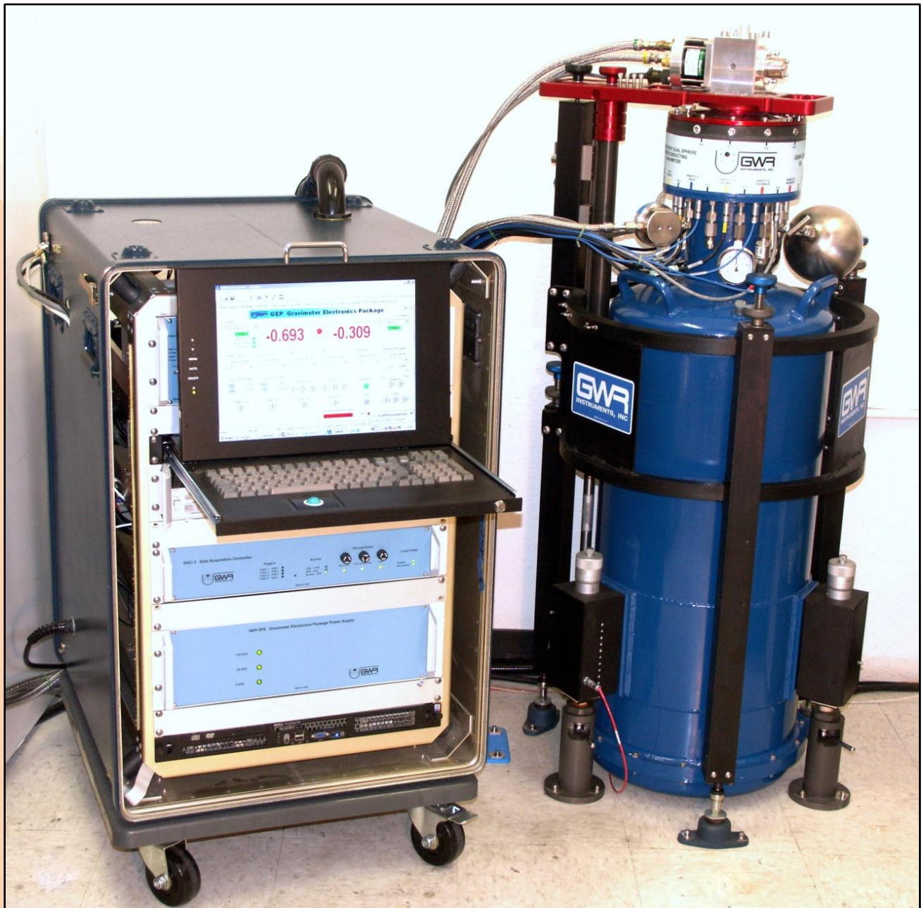
Observatory Superconducting Gravimeter (OSG), electronics package and 4K refrigeration system shown above
