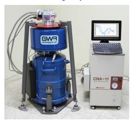
The iGrav SG provides continuous high-precision gravity data for studying a wide variety of geophysical phenomena
