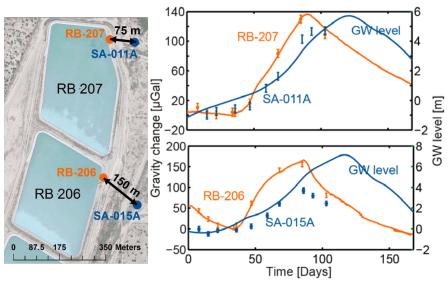
pond RB 206 500 m to the south. Extensive AG measurements (orange points with error bars) verify the drift-free operation of both *i*Grav SGs. Blue lines show ground water level for wells SA-011A and SA-015A; blue points and error bars are co-located AG measurements. These data show how gravity variations can vary dramatically at an active hydrological site over short times and short spatial distances.
